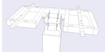
Make sure to run the two cables exiting the column through the cut out of the board frame before securing the 4 bolts.
